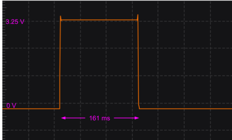
Figure 4. Oscilloscope trace of output when pushbutton is quickly pressed and released
