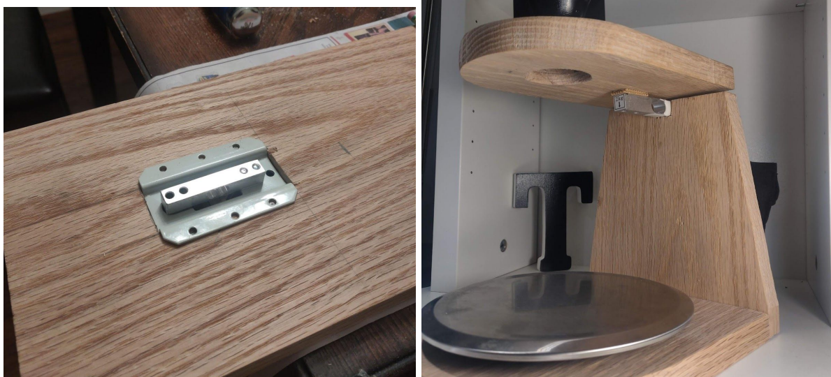
Bottom and Top Load Cell Mounting
