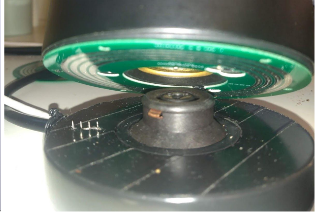
PCB and spring pin interface
