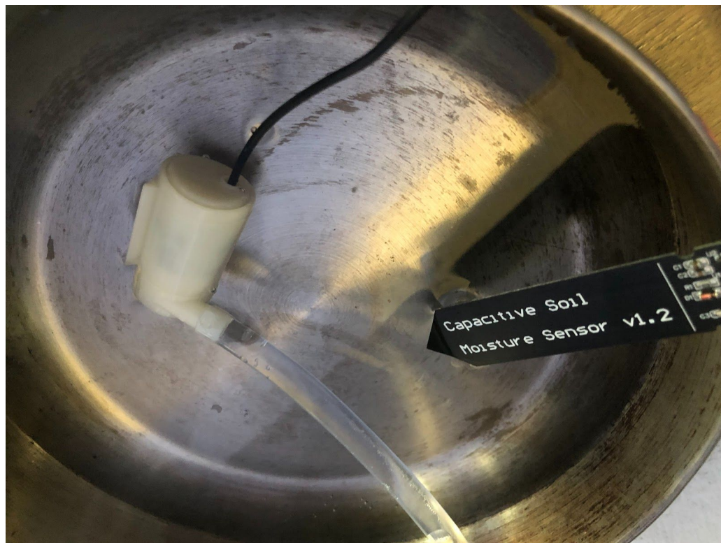
Figure 2. Pump and Sensor
