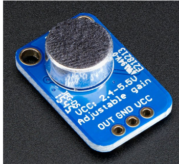
Figure 3: Electret microphone with amplifier (ADA 1063) [4]
