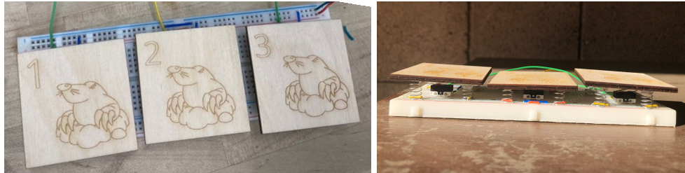
Figure 5. Finished Whack-A-Mole board with laser-etched platforms and spring setup.
