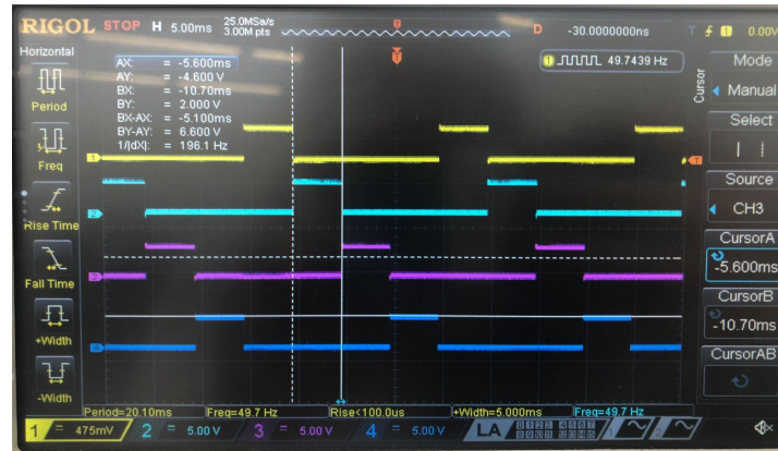
Figure 7. Logic Analyser of Stepper Motor Signals
